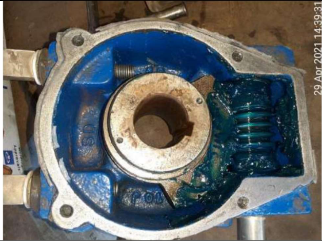
No water ingress found after immersion test of gearbox under 3 meter headpipe
