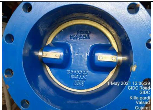
Solution test – internal valve visual inspection after 48 hours
