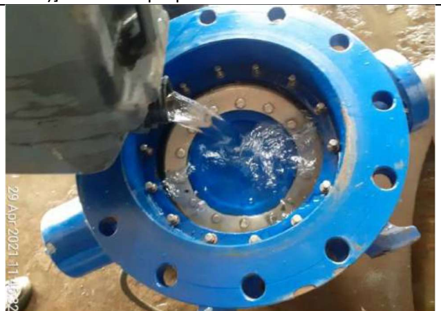
Solution test – internal valve visual inspection after 48 hours
